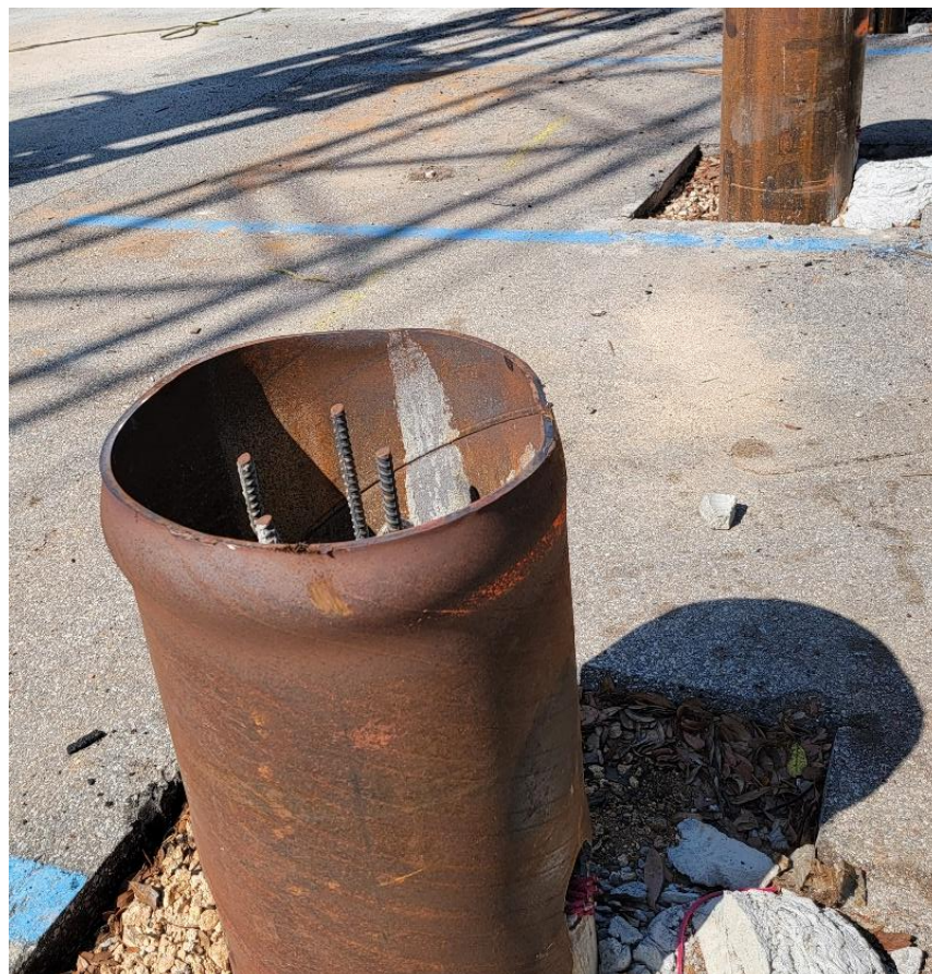
Figure 4. Deformed pile head of TP3 during second restrike test
