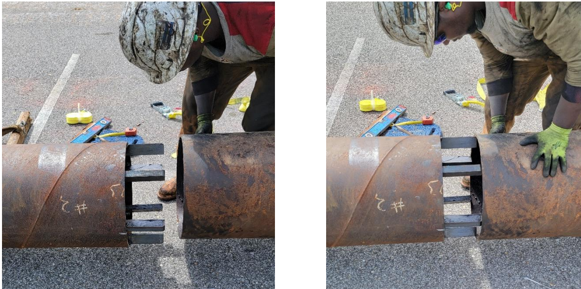
Figure 20. Pile TP5 splice for bidirectional testing
